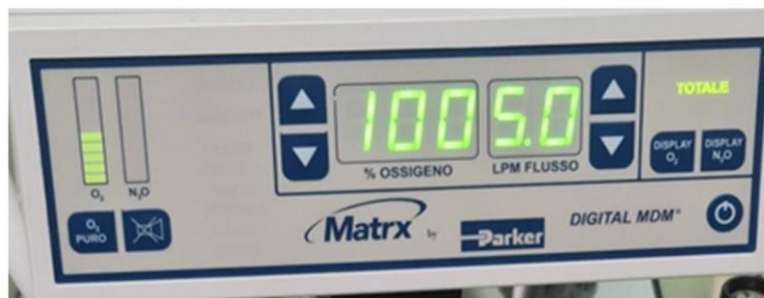
Fig. 3 Control panel that allows the flow rate of oxygen and nitrous oxide to be varied.
