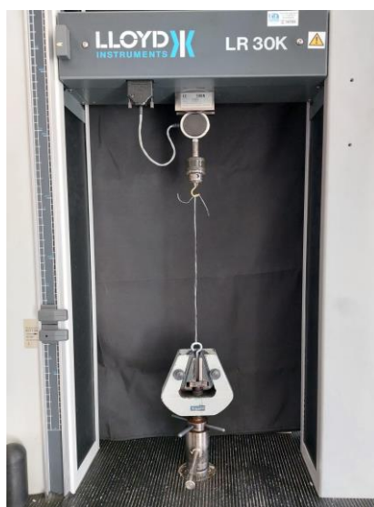
Fig. 1. Universal testing device Lloyd Instruments LR 30K Stress Test Machine (AMETEK® Test and Calibration Instruments).
