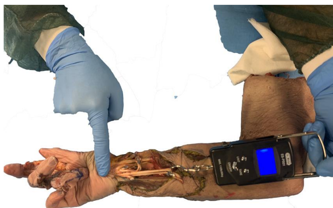
Fig. 3. The FDS and FDP tendons sutured side to side and attached to the S-shaped hook of the dynamometer.
