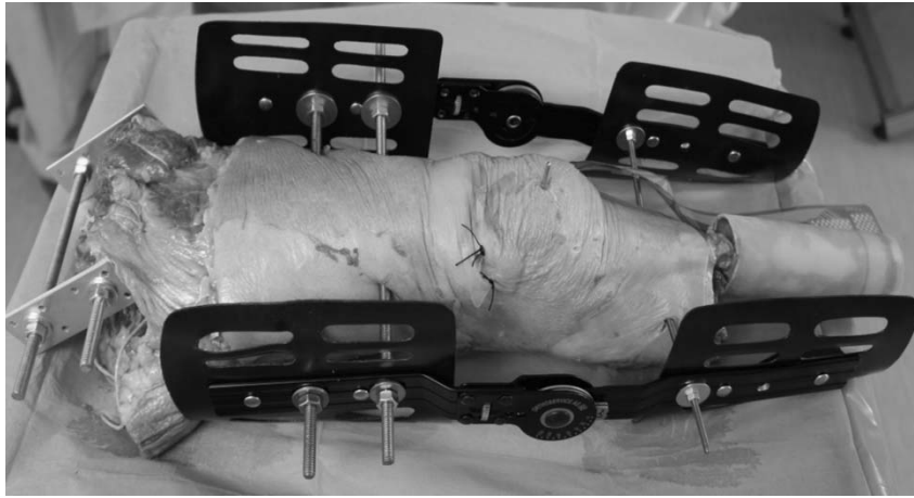
Fig. 2. The articulated frame fixed to the specimen. Metal rods are perpendicular to the mechanical axes, approximately 10 cm away by the joint line
